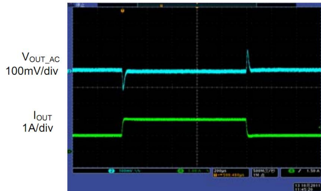
Fig. 11: Load transient ( I_{OUT}=1A to 2A ) Base Time 200\mu s/div
