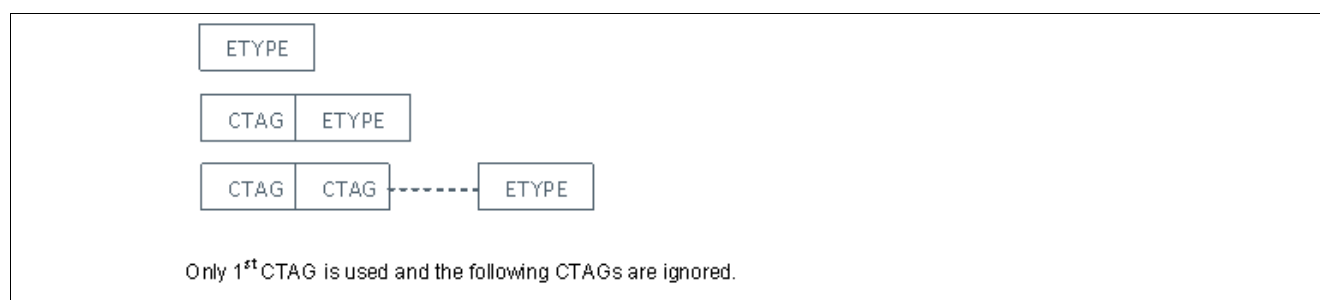
Figure 30 Supported Frame Formats when STAG is disabled
