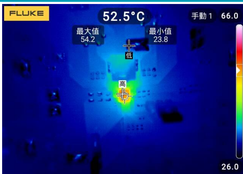
Thermal Image at V_{IN} = 15V, V_{BAT} = 8V, I_{CHG} = 2A
