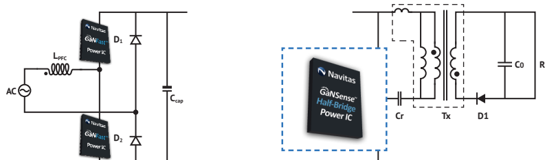
Fast Charger (Totem Pole + Asymmetric Half-Bridge) using GaNFast ICs and GaNSense Half-Bridge IC
