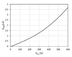
Fig. 10. Energy stored in output capacitance (E<sub>oss</sub>) vs. drain-to-source voltage (V<sub>DS</sub>)
