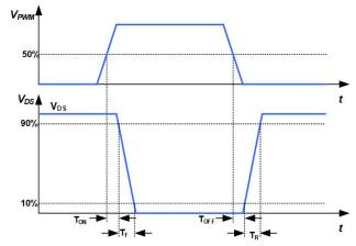
Fig. 2. Propagation delay and rise/fall time definitions
