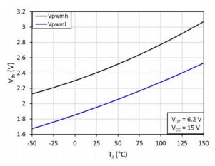
Fig. 7.  $V_{PWMH}$  and  $V_{PWML}$  vs. junction temperature(T<sub>J</sub>)
