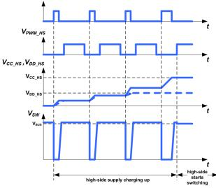
Fig. 20. ACF half-bridge start-up timing diagram
