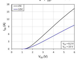
Fig. 5. Source-to-drain reverse conduction voltage
