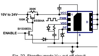
Fig. 22. Standby mode Vcc cut-off circuit
