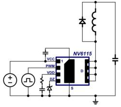
Fig. 1. Inductive switching circuit
