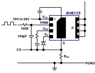
Fig. 24. Current sensing circuit
