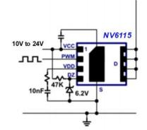
Fig. 27. Increasing Zener bias current for stable Zener voltage
