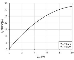
Fig. 3. Pulsed Drain current ( $I_D$  PULSE) vs. drain-to-source voltage ( $V_{DS}$ ) at T = 25 °C
