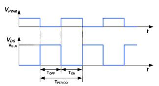
Fig. 21. Normal operating mode timing diagram
