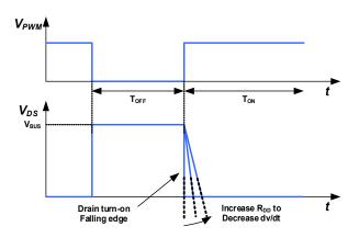
Fig. 23. Turn-on dV/dt slew rate control
