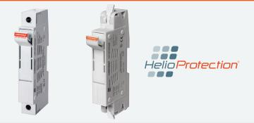
Mersen's 1500 VDC HelioProtection fuse holders for 10/14x85mm gPV fuses introduce the next level of safety for Utility scale photovoltaic applications. The HP15FHM32 fuse holders are finger safe (IP20 ingress protection rated), featuring a rotating fuse carrier, similar to the Mersen UltraSafe® fuse holders.
