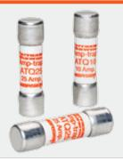
Amp-Trap® ATQ midget time-delay fuses are rated a full 500 volts AC with 42 ampere ratings from 1/10 to 30A. They are an excellent choice for supplemental protection of circuits up to 30A where the available short circuit current does not exceed 10,000A. (Not for Branch Circuit Protection).
