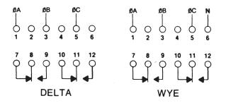
The **PBC Series** offers protection to three-phase equipment that is required to operate between two voltage limits. All three phases are monitored individually for a pre-selected **UNDER** and **OVER VOLTAGE** limit.
