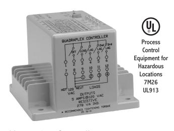
These **TRIPLEX** and **QUADRAPLEX CONTROLLERS** are available with either Sequence-On-Simultaneous-Off **(SOSO)** or First-On-First-Off **(FOFO)** output logic. The special function models are differentiated by a rotary switch that allows any output to be locked as the lead load or any one load to be omitted while sequencing only the remaining loads. In addition to load omission and lead selection, the expandable model can be set for 2, 3, or 4 load operation with either SOSO or FOFO logic.
