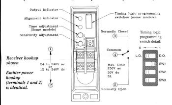
The output timing logic function (on sensor models with T9 model number suffix) is selected at the *timing logic programming switches*, according to the table (right). The output timing logic delays are set at
