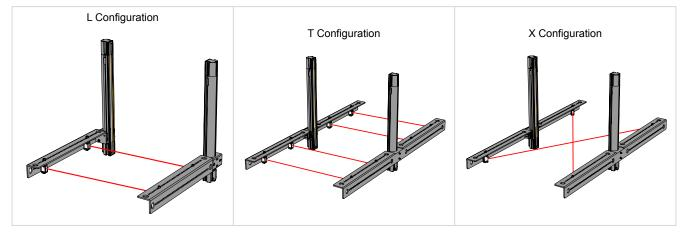
The S4B Mute Arm Sensor Kits can be directly mounted to a flat surface. The kits can also be mounted to the S4B Safety Light Curtain system's mounting brackets, S4BA-MBK-16 (or for the T and X system, directly to a stand). Connect the included Q20-2 sensors and the light curtains to the muting device. The use of an appropriate molded junction block, such as R95-6M125-M128-S4BM, can simplify wiring.
