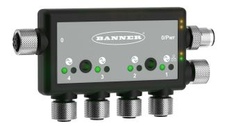
The DXMR90-4K contains four IO-link ports, allowing for concurrent communication to up to four IO-Link devices. Data is collected into the internal logic controller to facilitate edge processing, protocol conversion to Industrial Ethernet, Modbus/TCP, and pushing information to web servers. In addition to IO-Link devices, the IO-Link master can be used to transmit up to eight discrete signals using pin 2 or pin 4 of the IO-link master ports.
