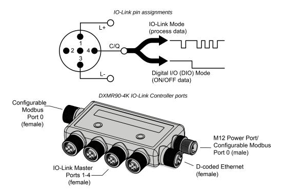
One male M12 connection provides common power and ground to all M12 IO-Link ports. One 100 Mbps Ethernet port (female) uses an M12 D-coded Ethernet connection.
