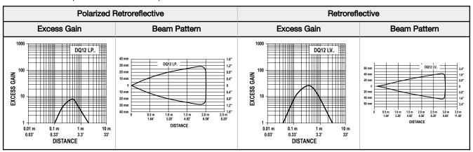
Fixed-field focus and spot sizes are typical. Performance based on use of 90% reflectance white test card.\*
