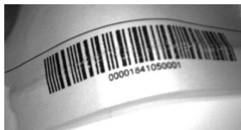
Figure 192. Barcode Printed on Curved Surface Readable by ABR in spite of Image Optical Distortion
