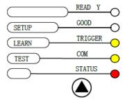
Step 4. The scanner is programmed and the AutoLearn Mode ends. The green "ready" LED is on.
