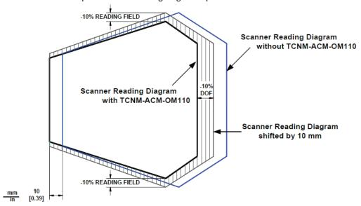
The reading distance also depends on the amplitude of aperture used. In particular, wider apertures require the scanner to be closer to the code in order to read at the extreme edges of the sweep (see figure below).
