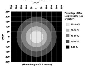
Lux and irradiance values shown are typical at 25 °C and with clear windows; light intensity lowered by 40% on diffuse window models.
