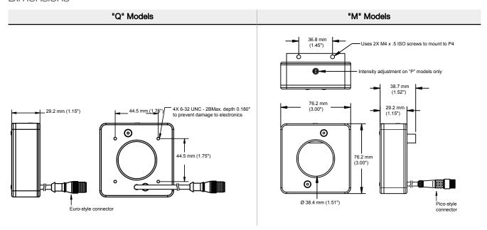
All measurements are listed in millimeters [inches], unless noted otherwise.
