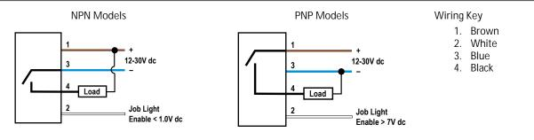
Note: Cabled wiring diagrams are shown. Quick disconnect (QD) wiring diagrams are functionally identical.
