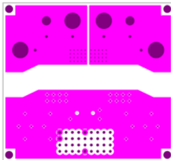
Figure 7. Board layout for measuring thermal resistance of CZ-3723
