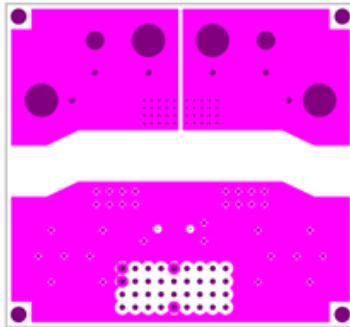
Figure 7. Board layout for measuring thermal resistance of CZ-3720
