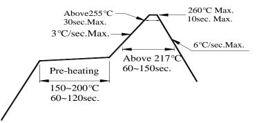
3.2 Reflow soldering should not be done more than two times.
