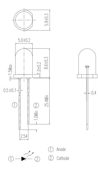
Note: Tolerances unless dimensions ±0.25mm
