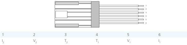
I: applied current V: measured voltage T: temperature sensor
