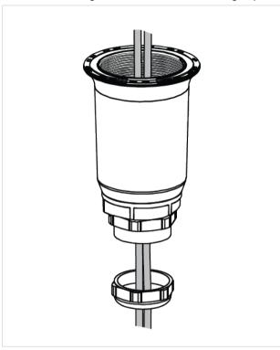
9. Pull the cables through the Bolt Base Protector and the cable gland parts.
