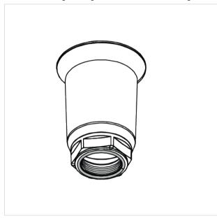
6. Attach the cable gland o-ring to the Bolt Base Protector bottom groove.
