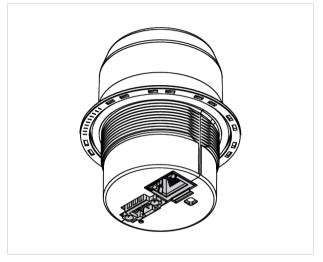
11. Attach the Bolt Base Protector to the Bolt.
