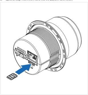
2. Optional step: Insert a SIM card into the **Bolt** SIM card holder.
