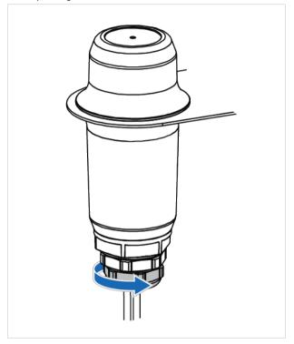
15. Check that the cable gland parts, the cable gland sealing insert and the cables are properly secured.
