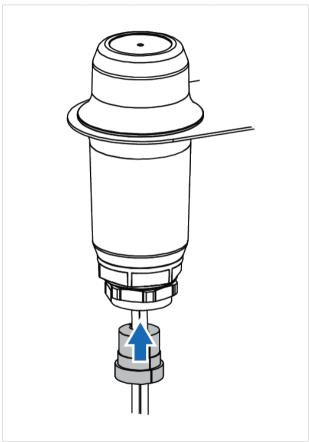
13. Attach the cable gland sealing insert to the cable gland top.
