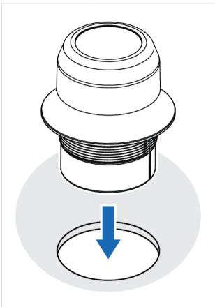
4. Place the Bolt in its mounting hole; in a surface or in the Bolt Bracket.
