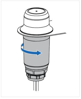
12. Open the slits and fit the cable gland sealing insert over the cables.
