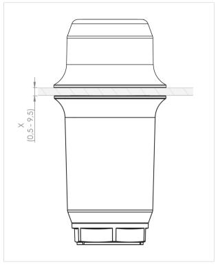
The thickness of the mounting surface must not exceed 10 mm.
