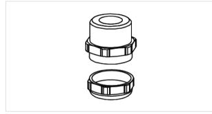
Attach the cable gland top to the Bolt Base Protector. Tightening torque: 5 Nm
