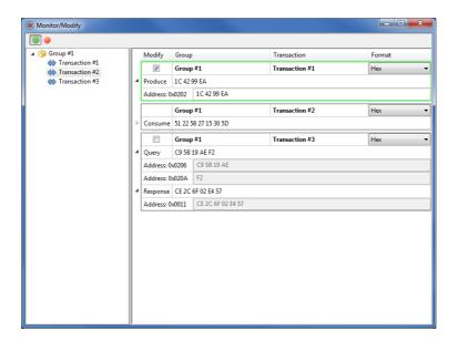
If Modify is enabled, it is possible to change the data values during runtime in Produce transactions and in the Query part of Query/Response transactions, i.e. only the out area of the Communicator can be modified. This will inhibit any data from the industrial network (DeviceNet), but input data from the CAN network will still be updated.
