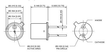
Note: Lead soldering temperature (1/16 inches from case) 260  $^{\circ}$ C for 3 sec.
