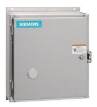
Electrically held lighting contactor, Contactor amp rating 60A, 0 N.C. / 6 N.O. Poles, 480VAC 60HZ coil, 1 NO / 1 NC auxiliary contacts Non-combination type, (no disconnect device), Encl NEMA type 4X 304 S-Steel, Water/dust tight noncorrosive
