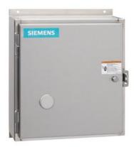
Electrically held lighting contactor, Contactor amp rating 60A, 0 N.C. / 3 N.O. Poles, 208VAC 50/60HZ coil, 1 NO / 1 NC auxiliary contacts Non-combination type, (no disconnect device), Encl NEMA type 4X 304 S-Steel, Water/dust tight noncorrosive
