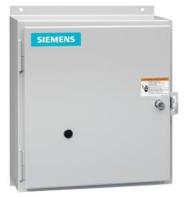
Electrically held lighting contactor, Contactor amp rating 60A, 0 N.C. / 6 N.O. Poles, 480VAC 60HZ coil, 1 NO / 1 NC auxiliary contacts Non-combination type, (no disconnect device), Enclosure NEMA type 12, Dust/drip proof for indoors
