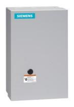
Electrically held lighting contactor, Contactor amp rating 60A, 0 N.C. / 12 N.O. Poles, 24VAC 50/60HZ coil, 1 NO / 1 NC auxiliary contacts Non-combination type, (no disconnect device), Enclosure NEMA type 1, Indoor general purpose use
