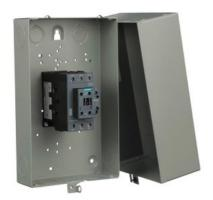
Electrically held lighting contactor, Contactor amp rating 60A, 0 N.C. / 3 N.O. Poles, 208VAC 50/60HZ coil, 1 NO / 1 NC auxiliary contacts Non-combination type, (no disconnect device), Enclosure NEMA type 1, Indoor general purpose use
