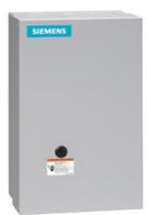
Electrically held lighting contactor, Contactor amp rating 30A, 0 N.C. / 9 N.O. Poles, 600VAC 60HZ coil, Non-combination type, (no disconnect device), Enclosure NEMA type 1, Indoor general purpose use
