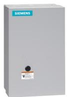
Electrically held lighting contactor, Contactor amp rating 30A, 0 N.C. / 6 N.O. Poles, 198VAC 50HZ/208VAC 60HZ coil, Non-combination type, (no disconnect device), Enclosure NEMA type 1, Indoor general purpose use
