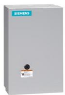
Electrically held lighting contactor, Contactor amp rating 30A, 0 N.C. / 6 N.O. Poles, 24VAC 50/60HZ coil, Non-combination type, (no disconnect device), Enclosure NEMA type 1, Indoor general purpose use
