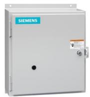
Electrically held lighting contactor, (convertible to mech. held), Amp rating 30A (tungsten 20A), 7 N.C. / 1 N.O. poles, 115-120V 60Hz/110V 50Hz coil, Noncombination type, Encl NEMA type 4X 304 S-Steel, Water/dust tight noncorrosive
