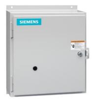
Electrically held lighting contactor, (convertible to mech. held), Amp rating 30A (tungsten 20A), 6 N.C. / 6 N.O. poles, 460-480V 60Hz/440V 50Hz coil, Noncombination type, Encl NEMA type 4X 304 S-Steel, Water/dust tight noncorrosive
