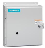
Electrically held lighting contactor, (convertible to mech. held), Amp rating 30A (tungsten 20A), 4 N.C. / 0 N.O. poles, 115-120V 60Hz/110V 50Hz coil, Non-combination type, Encl NEMA type 4X 304 S-Steel, Water/dust tight noncorrosive
