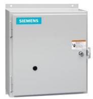
Electrically held lighting contactor, (convertible to mech. held), Amp rating 30A (tungsten 20A), 2 N.C. / 4 N.O. poles, 24V 60Hz / 20V 50Hz coil, Non-combination type, Encl NEMA type 4X 304 S-Steel, Water/dust tight noncorrosive
