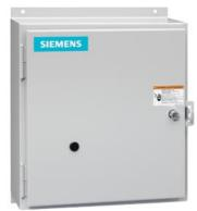
Electrically held lighting contactor, (convertible to mech. held), Amp rating 30A (tungsten 20A), 2 N.C. / 2 N.O. poles, 277V 60Hz / 240V 50Hz coil, Noncombination type, Encl NEMA type 4X 304 S-Steel, Water/dust tight noncorrosive
