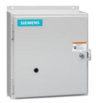
Electrically held lighting contactor, (convertible to mech. held), Amp rating 30A (tungsten 20A), 2 N.C. / 0 N.O. poles, 200-208V 60Hz coil, Non-combination type, Encl NEMA type 4X 304 S-Steel, Water/dust tight noncorrosive
