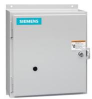
Electrically held lighting contactor, (convertible to mech. held), Amp rating 30A (tungsten 20A), 1 N.C. / 6 N.O. poles, 575-600V 60Hz/550V 50Hz coil, Non-combination type, Encl NEMA type 4X 304 S-Steel, Water/dust tight noncorrosive
