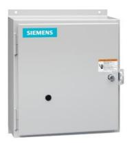
Electrically held lighting contactor, (convertible to mech. held), Amp rating 30A (tungsten 20A), 4 N.C. / 7 N.O. poles, 460-480V 60Hz/440V 50Hz coil, Noncombination type, Enclosure NEMA type 12, Dust/drip proof for indoors
