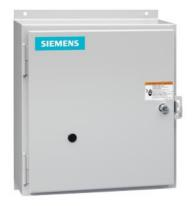
Electrically held lighting contactor, (convertible to mech. held), Amp rating 30A (tungsten 20A), 4 N.C. / 5 N.O. poles, 200-208V 60Hz coil, Non-combination type, Enclosure NEMA type 12, Dust/drip proof for indoors
