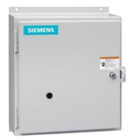
Electrically held lighting contactor, (convertible to mech. held), Amp rating 30A (tungsten 20A), 4 N.C. / 4 N.O. poles, 277V 60Hz / 240V 50Hz coil, Noncombination type, Enclosure NEMA type 12, Dust/drip proof for indoors
