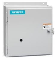
Electrically held lighting contactor, (convertible to mech. held), Amp rating 30A (tungsten 20A), 4 N.C. / 1 N.O. poles, 115-120V 60Hz/110V 50Hz coil, Non-combination type, Enclosure NEMA type 12, Dust/drip proof for indoors
