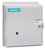
Electrically held lighting contactor, (convertible to mech. held), Amp rating 30A (tungsten 20A), 2 N.C. / 7 N.O. poles, 24V 60Hz / 20V 50Hz coil, Non-combination type, Enclosure NEMA type 12, Dust/drip proof for indoors
