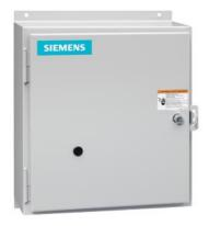
Electrically held lighting contactor, (convertible to mech. held), Amp rating 30A (tungsten 20A), 1 N.C. / 9 N.O. poles, 24V 60Hz / 20V 50Hz coil, Non-combination type, Enclosure NEMA type 12, Dust/drip proof for indoors
