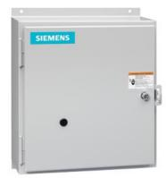
Electrically held lighting contactor, (convertible to mech. held), Amp rating 30A (tungsten 20A), 1 N.C. / 8 N.O. poles, 277V 60Hz / 240V 50Hz coil, Noncombination type, Enclosure NEMA type 12, Dust/drip proof for indoors
