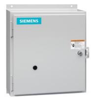
Electrically held lighting contactor, (convertible to mech. held), Amp rating 30A (tungsten 20A), 1 N.C. / 8 N.O. poles, 200-208V 60Hz coil, Non-combination type, Enclosure NEMA type 12, Dust/drip proof for indoors
